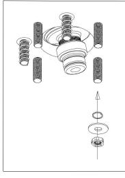
**STEP 2)** Slide 1 washer (B) followed 1 lock washer (A) and a nut (C) onto bolt connected to the sink (2).
